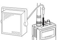
**Note:** You must use an amplified speaker with this scanner. Non-amplified speakers do not provide sufficient volume for comfortable listening.
